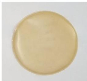
Gambar 3. Hasil Sintesis Membran *Chitosan*
