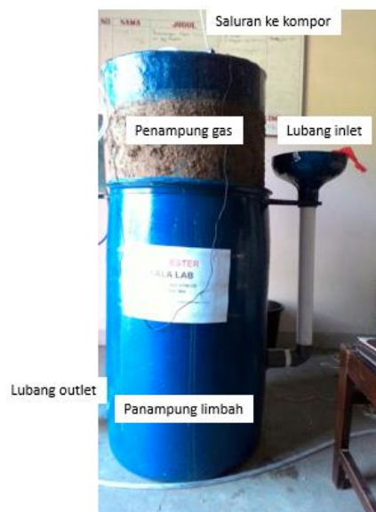
Gambar 2. Reaktor biogas tipe floating drum
