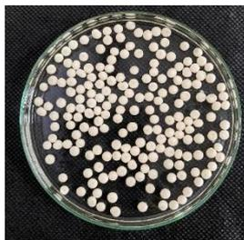
Gambar 5. Hasil Sintesis *Beads Chitosan – Clay*
